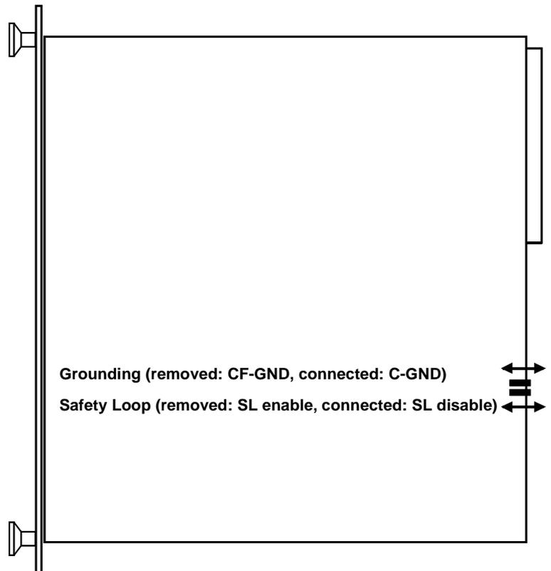
The shield is connected with the Crate-GND
