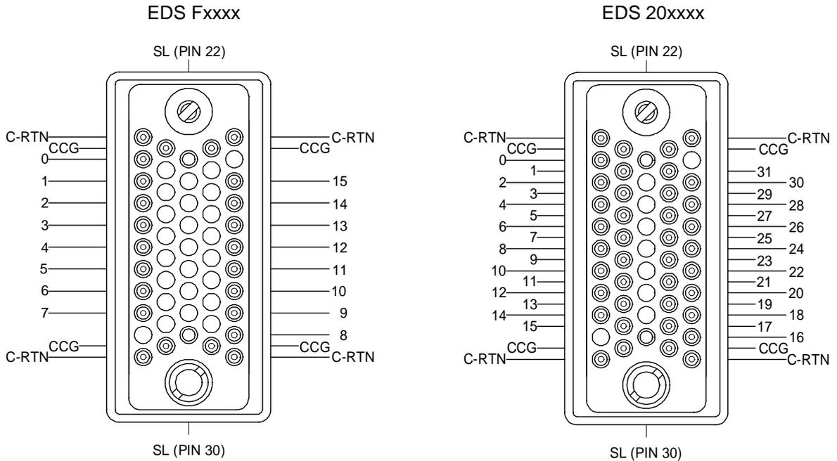
CCG is connected with the Crate-GND and the shield
