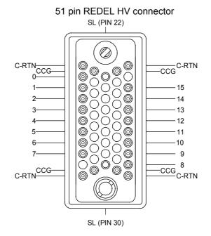
CCG is connected with the Crate-GND and the shield
