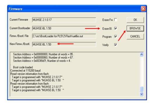
When the install process is done hit the button "cancel" to restart the system. It is recommended to close the muhse control program before restarting.
