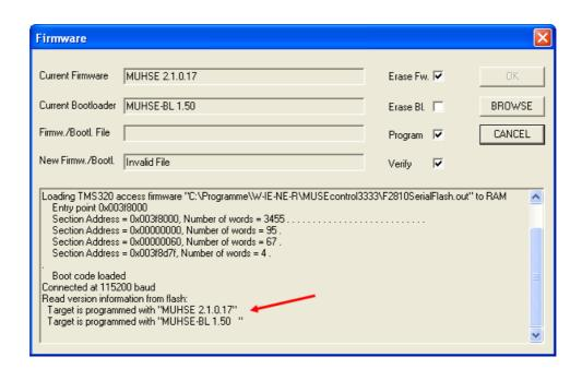
Option 1) Check "Erase Fw." (erase firmware) and "Erase Bl." (erase bootloader) if the current firmware is older than 2.\*.0.15 or it is a firmware without bootloader. After that push the button "browse" to scan the flash. In some minutes select the new bootloader file in the automatically opened file menu. Press the button "Ok". Now the whole flash will be erased and the new bootloader will be installed.
