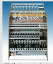
CERN LHC special crate, rear view with multiple transition card cages
