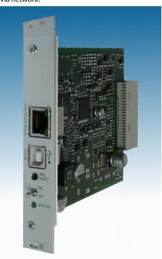
All necessary functions are implemented on a small (100 mm x 120 mm) board. The system connections are provided on a 2mm high density connector
