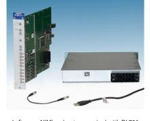
Left: open NIMbox (custom version) with DL706 main board and 4 submodules plugged in. Right: NIMbox rear side with USB port and NIM connector
