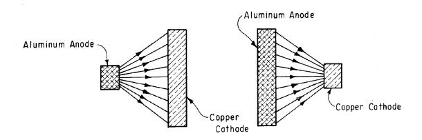
Figure 1. - Electrolytic current density diagram.
