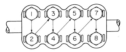
Figure 2. - Clamp tightening sequences.
