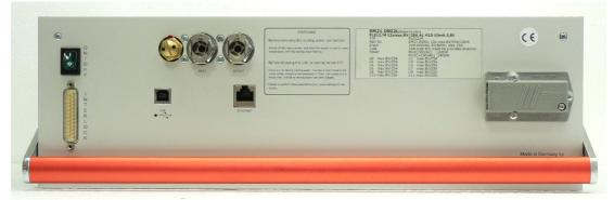
Figure 2.1: PL512 Front Side with Interlock and Water-Cooled Option
