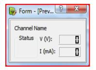
• Compact Voltage display widget which shows only voltage and current for a generic channel ("Channel Name" is replaced on instance init, with the EPICS channel name)
