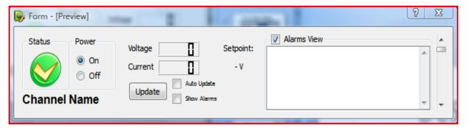
• The "detailed" voltage monitoring widget which includes a nice graphic status display, power indicator (not a control), a readback for both voltage and current, and a window showing a simple alarm history
