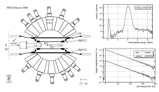
Fig. 1. Left: Cross section drawing of the PEN detector system. Right: Energy distribution of the intermediate muon in the  $\pi \rightarrow \mu \rightarrow e$  decay chain, extracted from AT waveform data (top). Time dependence of the  $\pi \rightarrow \mu$  and  $\pi \rightarrow e$  decays, from the AT waveform data.
