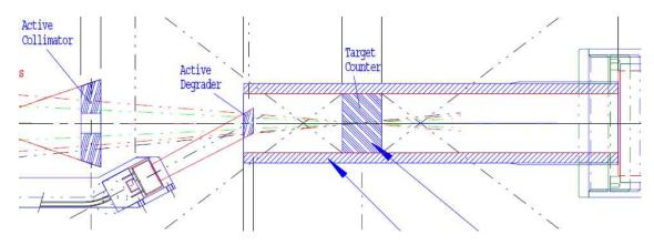
Figure 1: Schematic drawing of the central-region beam detectors redesigned for the 2006 PEN run: the active collimator, degrader, active target (with fast central scintillator and a slow-scintillator cylindrical shield). The upstream Beam tag detector, also redesigned for 2006, is not shown.
