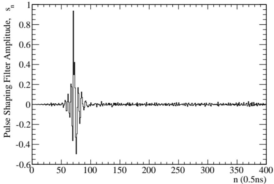
Figure: Pulse Shaping Filter.
