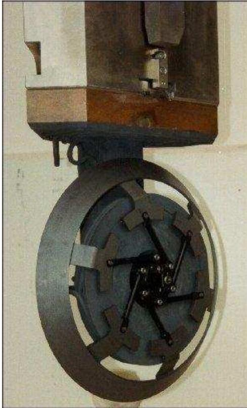
**Figure 3.2:** *The graphite pion production target [2].*
